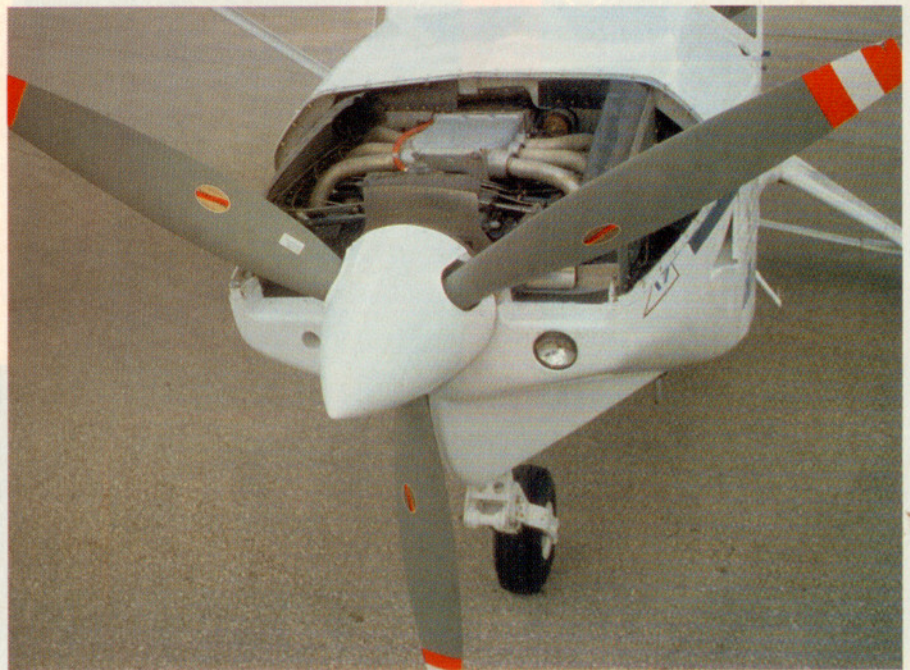
At 10,000 feet, the 350-horsepower Lycoming TIO-540 can pull the Gavilan through the air at 130 knots on 19 gallons per hour.
